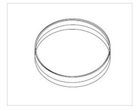
Dish height 14.5 mm, dish diameter 86.5 mm, wall thickness 1 - 1.2 mm
